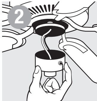
Remove switch housing cover and light kit if present.
